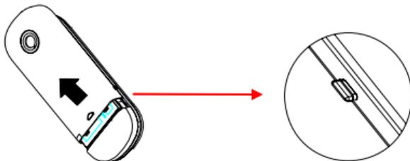
2. With the metal contacts facing into the phone clip the battery in place, positioning the bottom of the battery first.
